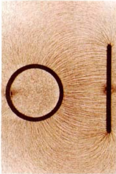
Electric field lines for an oppositely charged cylinder and plate, shown by bits of fine thread suspended in oil. Note that the field lines are perpendicular to the conductors and that there are no lines inside the cylinder.
