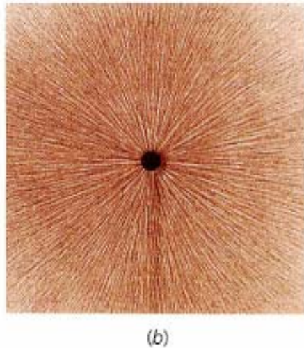
FIGURE 21-19 (a) Electric field lines of a single positive point charge. If the charge were negative, the arrows would be reversed. (b) The same electric field lines shown by bits of thread suspended in oil. The electric field of the charged object in the center induces opposite charges on the ends of each bit of thread, causing the threads to align themselves parallel to the field.
