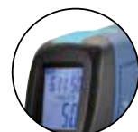
Normal Temperature with Green LED indicator
