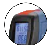
Higher temperature Located with Red LED indicator
